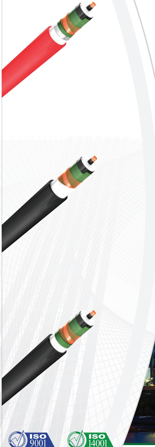
Power cables with copper or aluminium conductors, extruded XLPE insulation sheathed with PE (PVC) outer sheath for rated voltage above 36 kV up to 420 kV. For supply of electrical energy, laying in ground, ducts, pipes and air.
