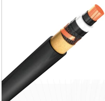
Cables for electric current transmission at distribution network, at distribution industrial plant, thermo and hydroelectric plants etc. Nominal voltage: up to 35 kV.
